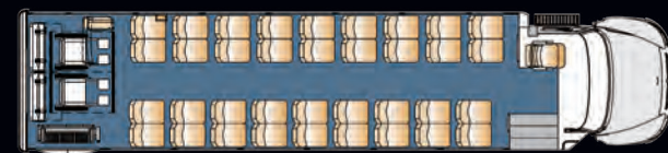
36 Passenger Plus 2 Wheelchair Positions Plus 2-Passenger Foldaway and Two 2-Passenger Flipseats
